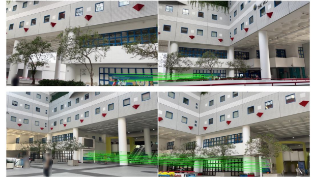
Fig. 10. Example visualisations of keypoint matching between a query image (left) and database image(right) in AnchorLoc. Using the information from the detected anchor, AnchorLoc can boost the localisation efficiency by limiting the search space during image retrieval and reducing the number of processed keypoints during pose estimation.
